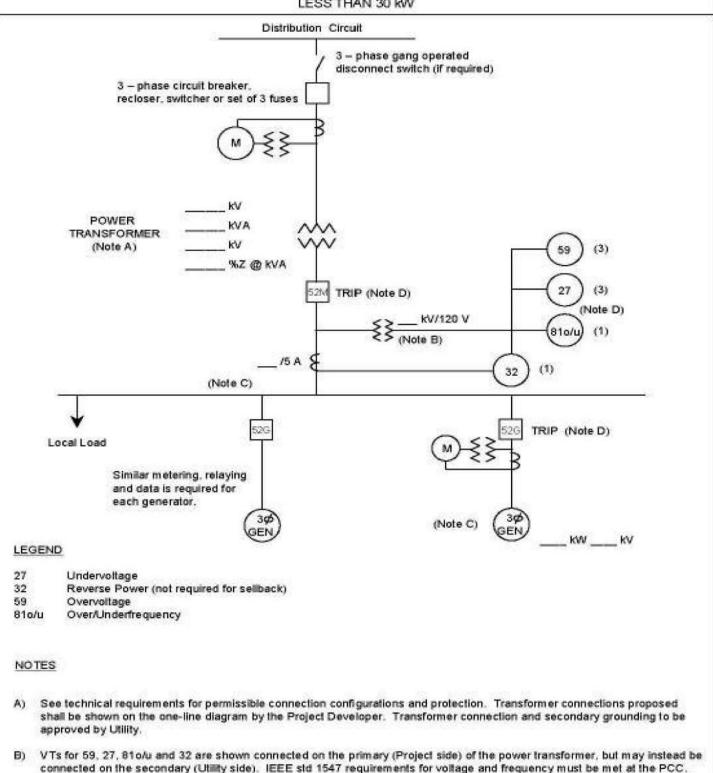
C) Main breaker protection, generator protection and synchronizing equipment are not shown.
