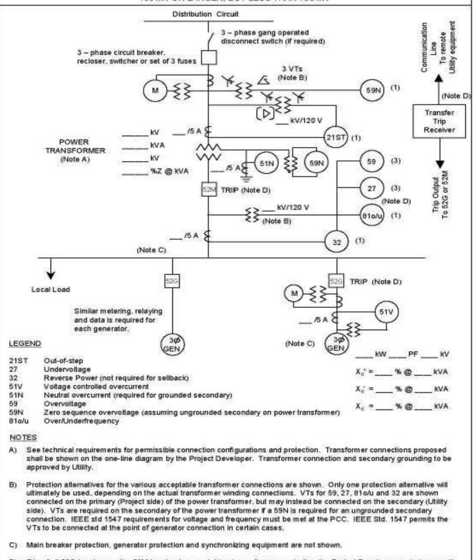
D) Trip of all 52G breakers or the 52M breaker is acceptable, depending upon whether the Project Developer wants to serve its own isolated load after loss of Utility service.
