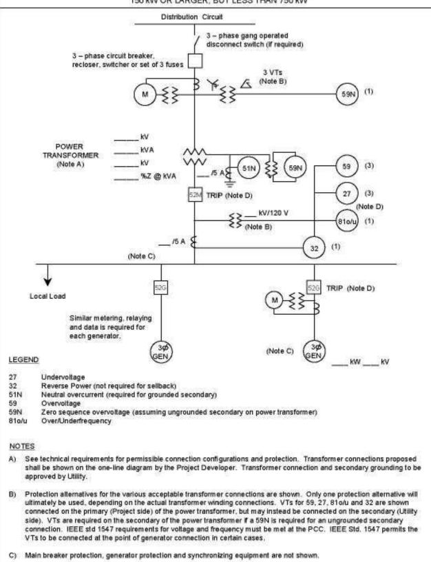
D) Trip of all 52G breakers or the 52M breaker is acceptable, depending upon whether the Project Developer wants to serve its own isolated load after loss of Utility service.
