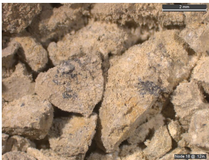
Fig. 6 Node 18 12 in. – Dark patches are CCR embedded in clay.
