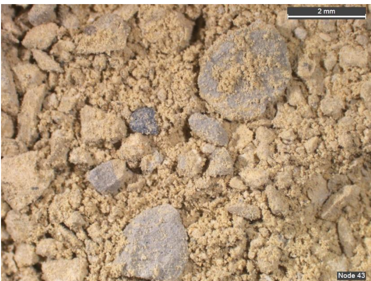
Fig. 2 Node 43 – The dark particle is CCR. The sample mainly consists of yellow clay and pale gray clay.
