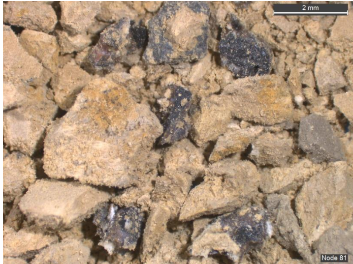
Fig. 4 Node 81 – Dark particles are CCR. The sample mainly consist of buff, yellow, and pale gray clay.
