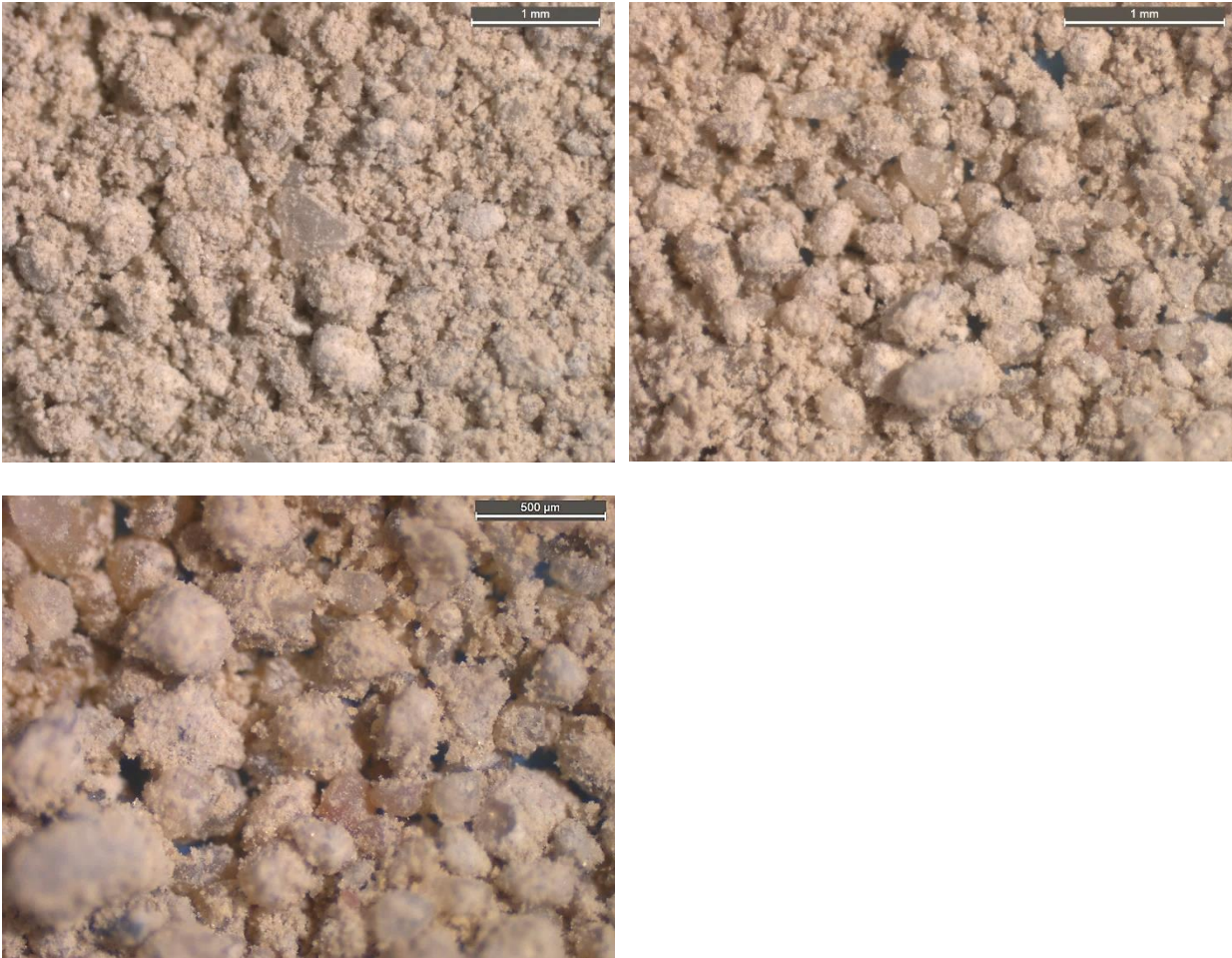
Fig. 2 Granular Material in Clay Soil Sample U3E-CS-03. The soil sample consists of powder and granules of quartz, feldspar, and granite. The area photographed was intentionally selected to illustrate the granular particles and does not represent the overall abundance of these particles in clay soil sample.
