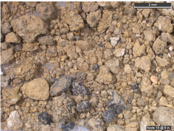
Fig. 5 Node 18 6 in. – Dark particles are CCR. The sample mainly consists of yellow clay and pale gray clay.
