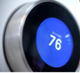
The thermostat stores the set point and schedule. When power is lost to the thermostat, the only information it "loses" is the current time. Once power is restored, the
